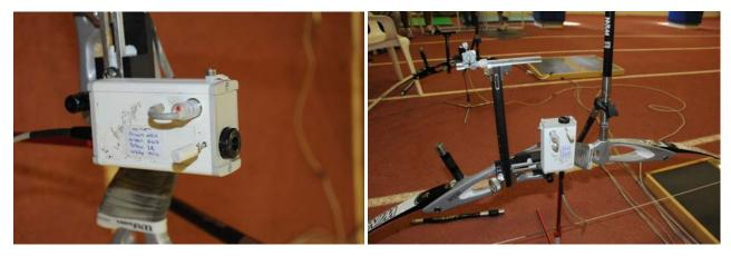
Picture 2. Detector of clicker drop sound and infrared beamer box attached on a bow.
